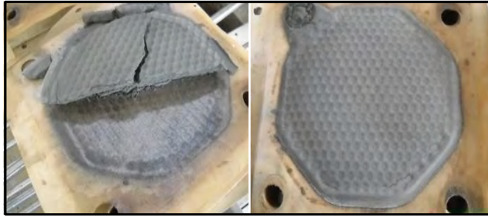
Figure 13-29: Filtration Cakes – Non-Magnetic Tailings (12.6% w/w Moisture)
