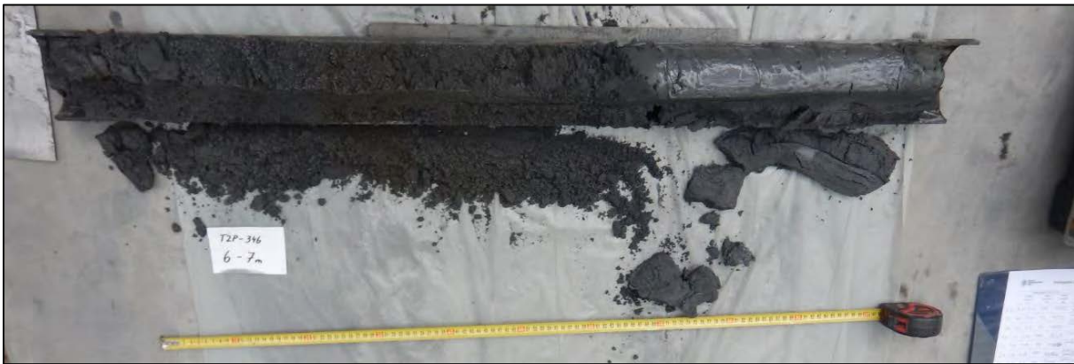
Figure 12-2: View of 1 m Tailings Core Being Quarter Split (uphole direction is to right), T2P-346, 6-7m
