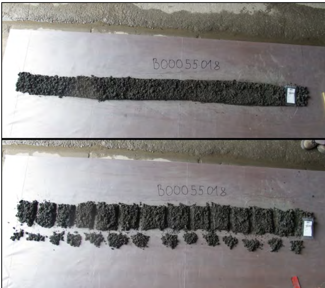
Figure 11-6: Example of Sample Splitting by the Wet Japanese Slab Cake Homogenization Method
