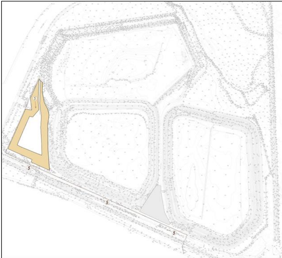
Picture no. 7: Temporary deposit of overburden material from the plant construction area
