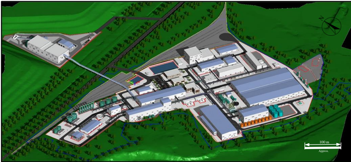
Figure 1-7: Preliminary Process Plant Site Layout (3D Format)
