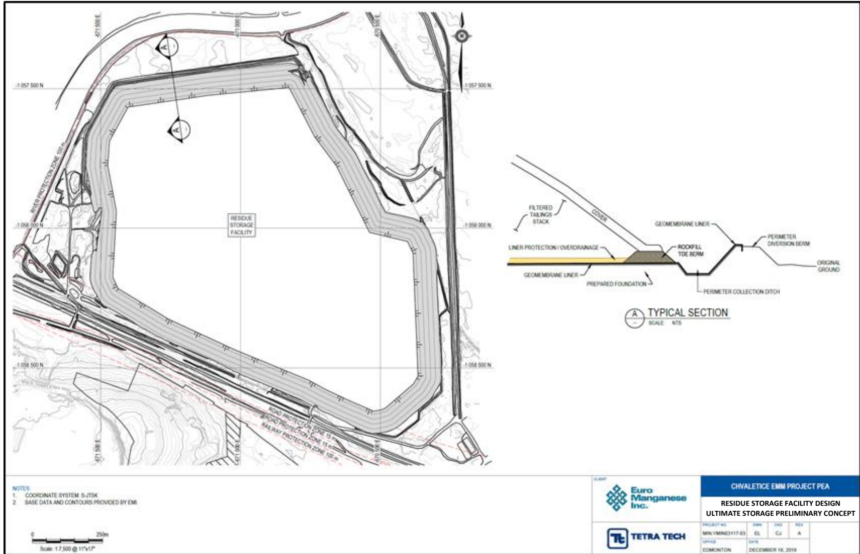
Figure 1-7: RSF Design Ultimate Storage – Preliminary Concept (Final design subject to community and regulatory consultation)
