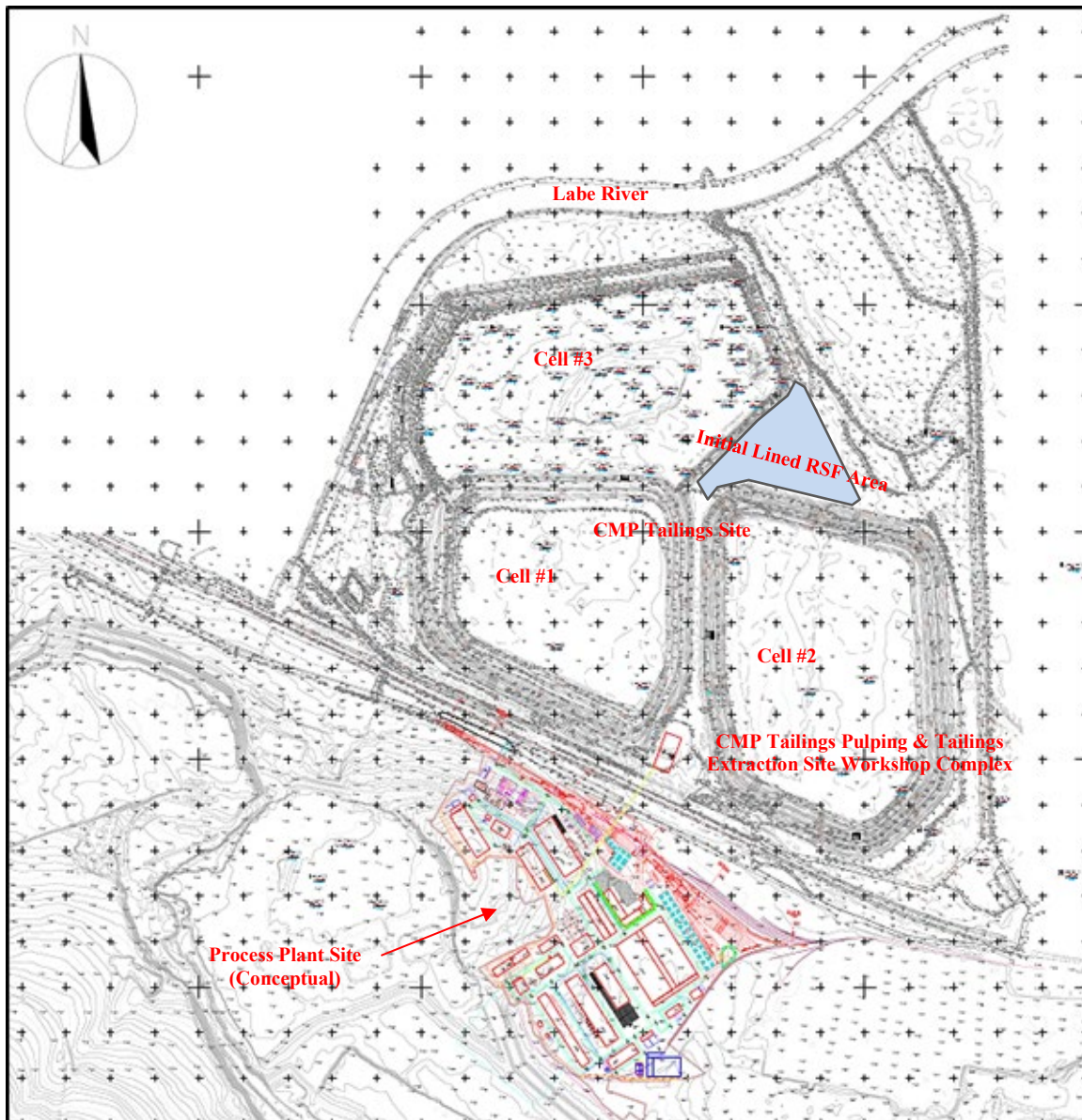
Figure 1-5: CMP Project Site Layout
